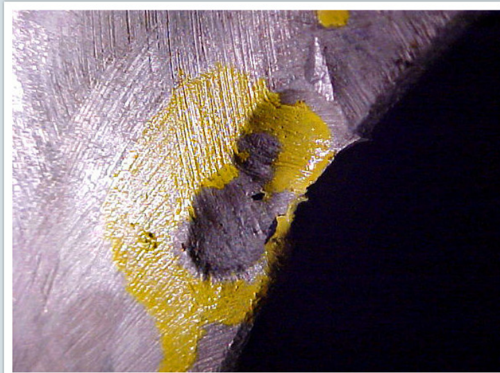
PHOTO #5 Pinhole Porosity Defect
